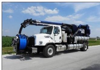
Vactor truck that cleans storm drains
